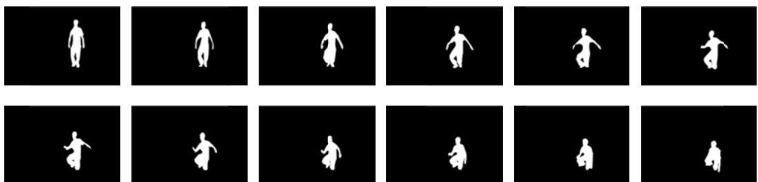
Figure 4-17: The object masks of falling behavior performed by person 2 and captured from the front side.
